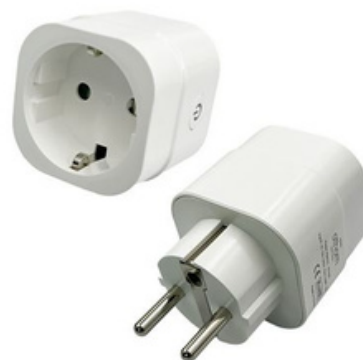
Smart plug with Tasmota firmware
